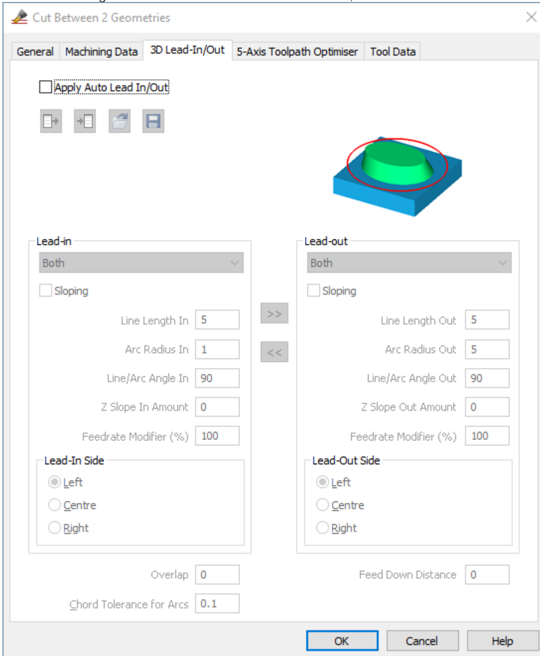
Figure 92 - Cut Between 2 Geometries 3D Lead-In/Out tab
