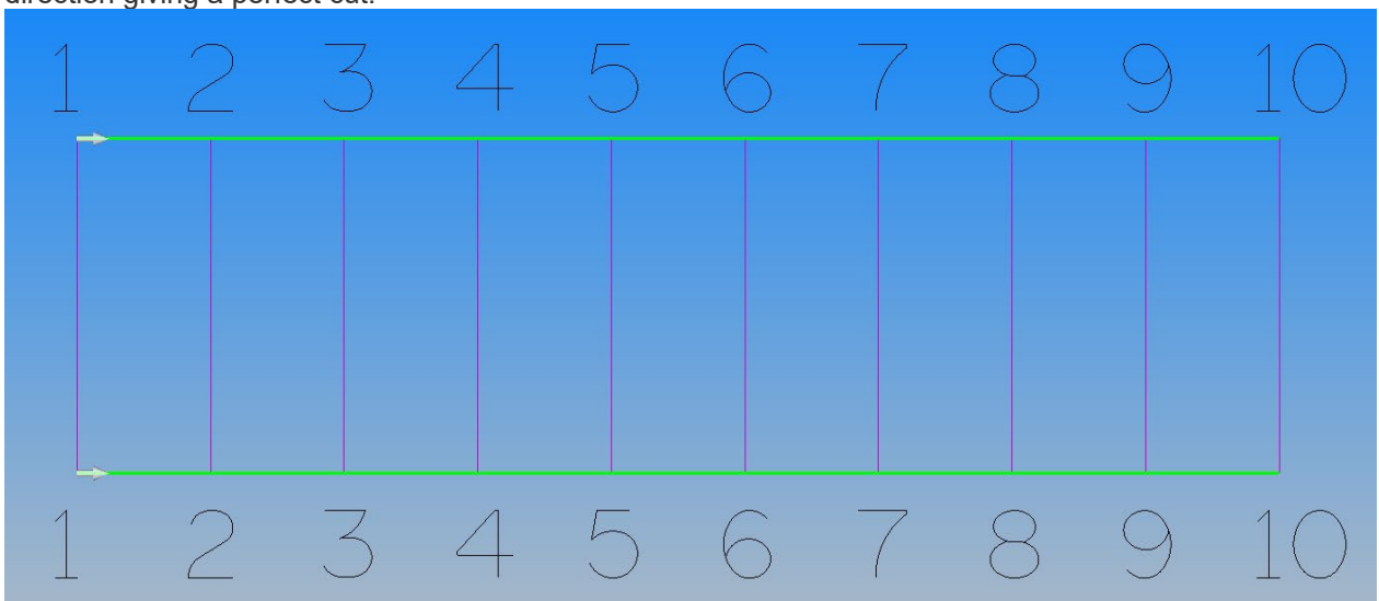
Figure 48 - How point matching works when lines are set correctly
