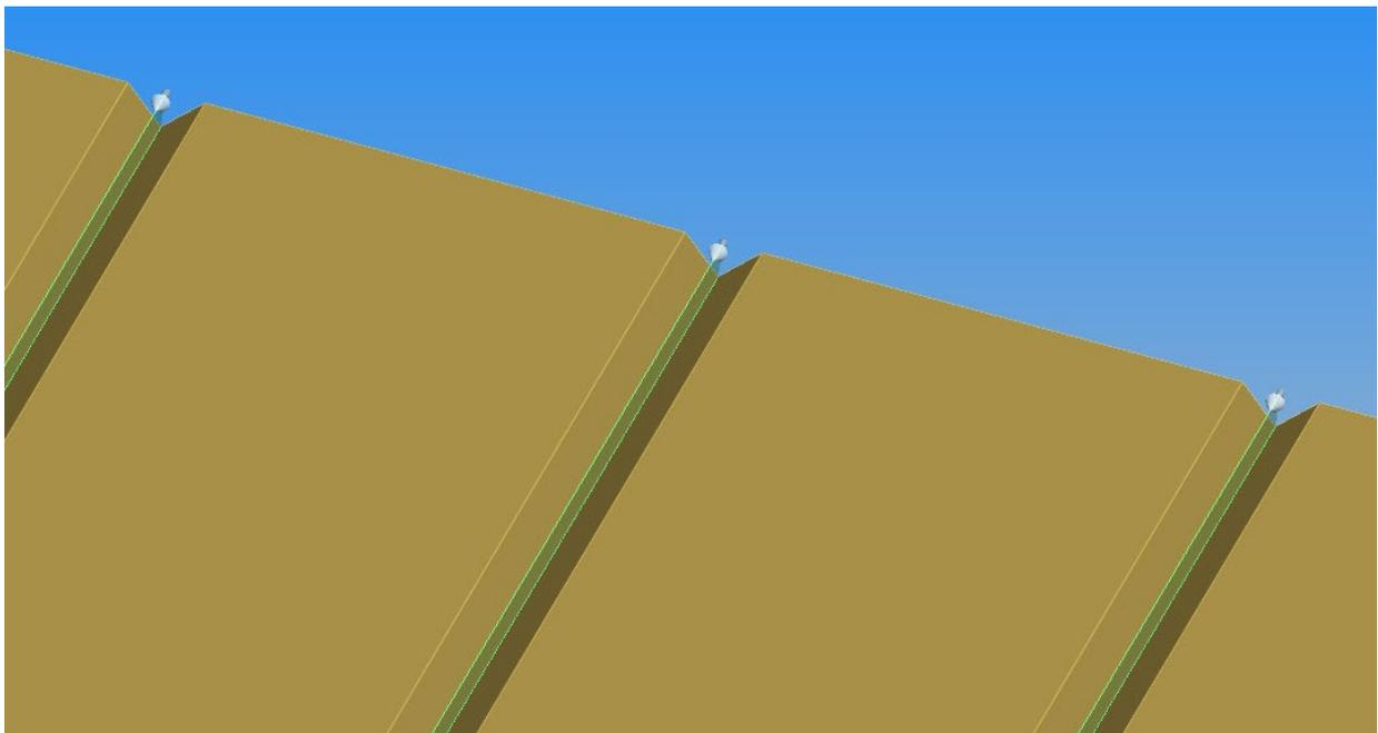
Figure 131 - V-slots correct for manufacture
