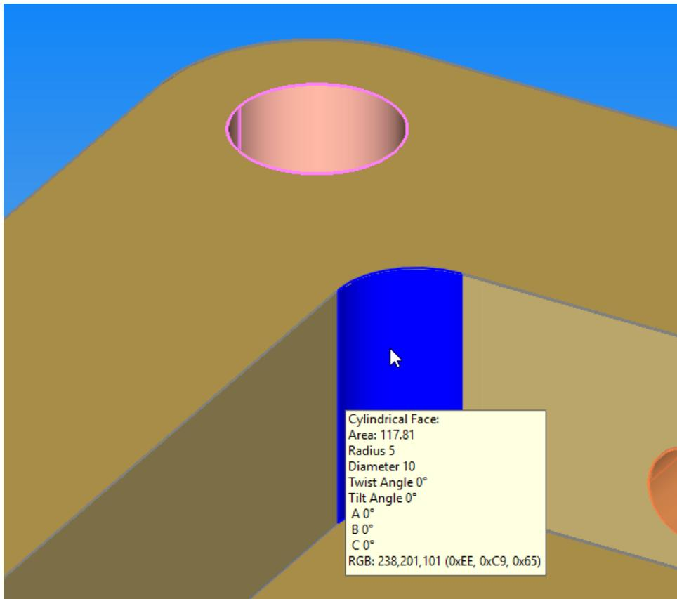
Hovering over an internal fillet radius to see what size tool is required.
