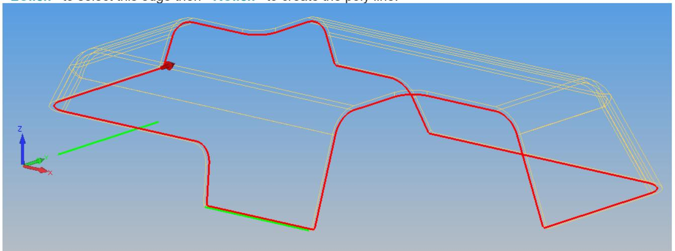
Figure 210 - 3D Edge Extraction seen in unshaded mode
