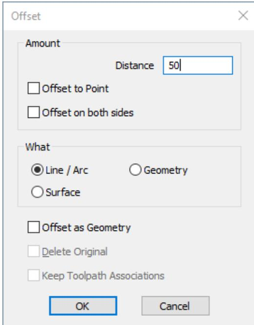
Figure 108 - Offset options for the guide line
