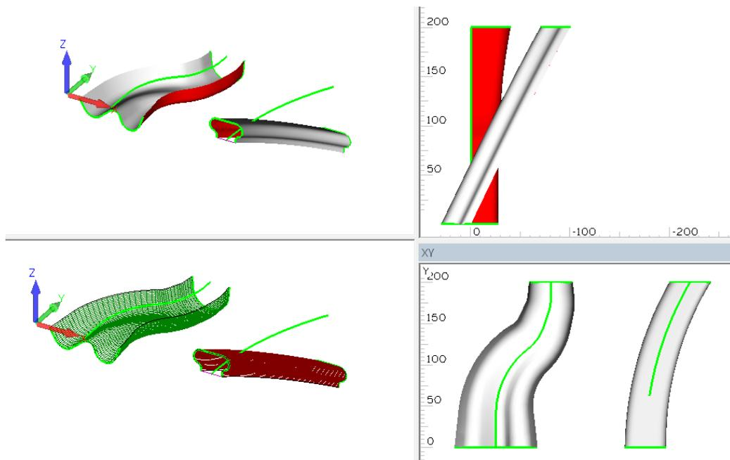
Figure 31 - Swept Surface 3 Curves completed examples
