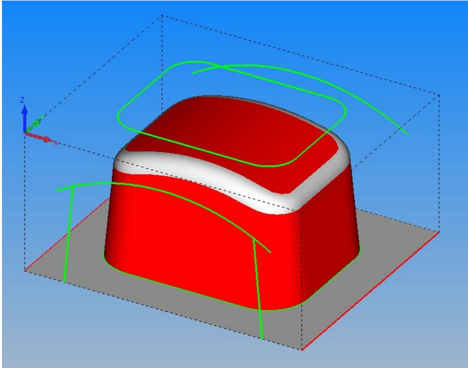
Figure 95 - Complete applied fillet surface
