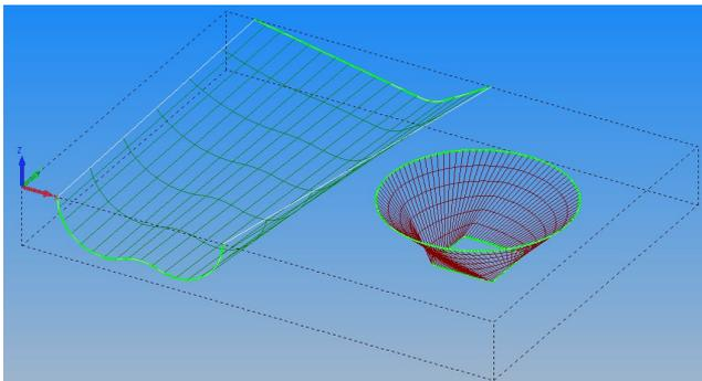
Figure 24 - Ruled surfaces created and viewed in wireframe and shaded
