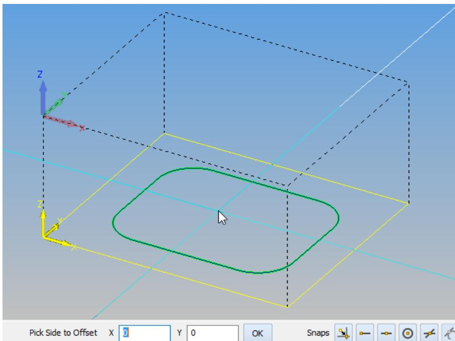
Figure 50 - Apply the Offset to the inside
