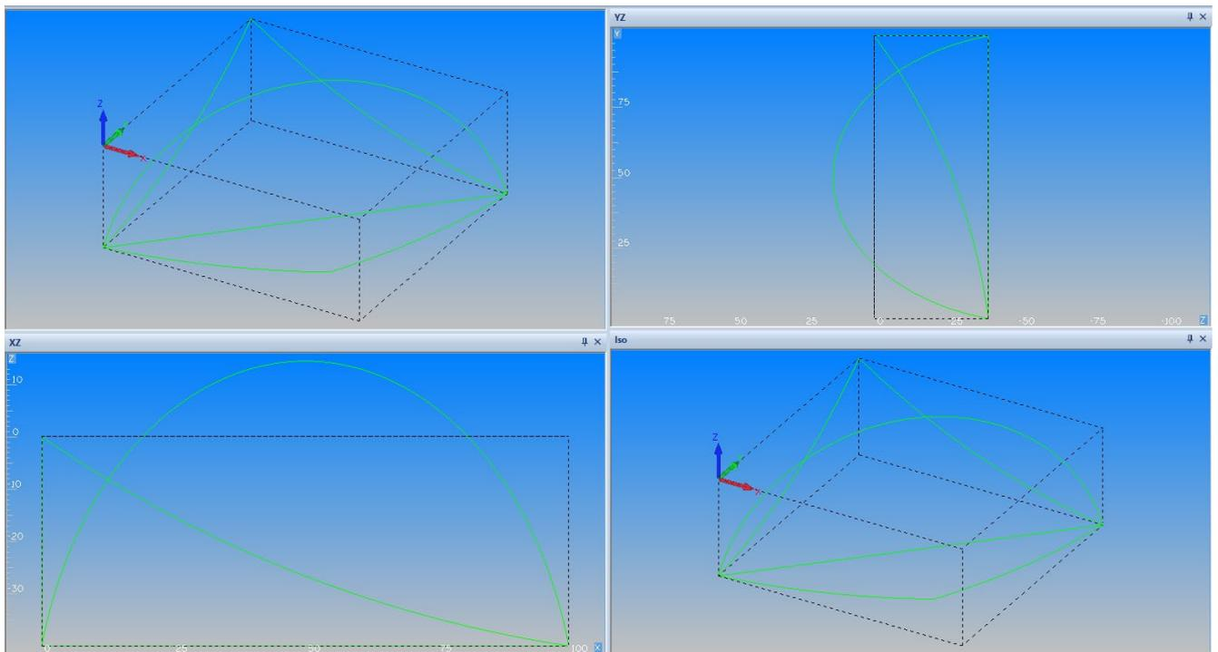
Figure 35 - Coons Patch example drawing
