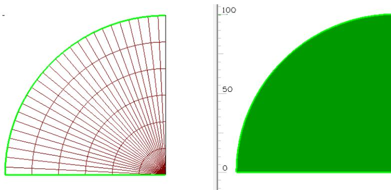
Figure 26 - Straight line sweep with rotation
