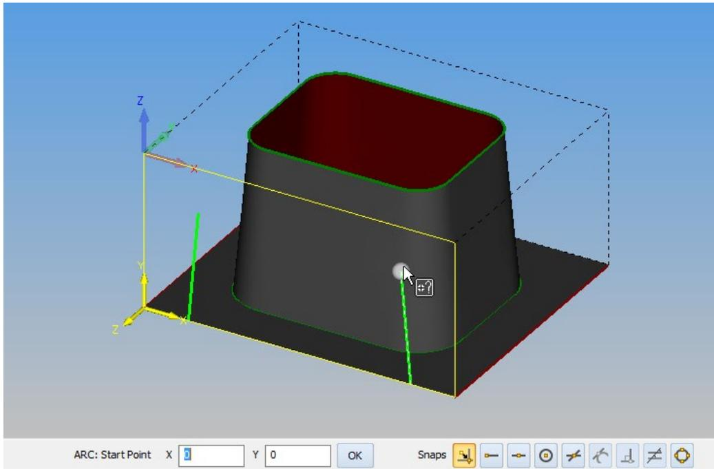
Figure 75 - First point of the arc
