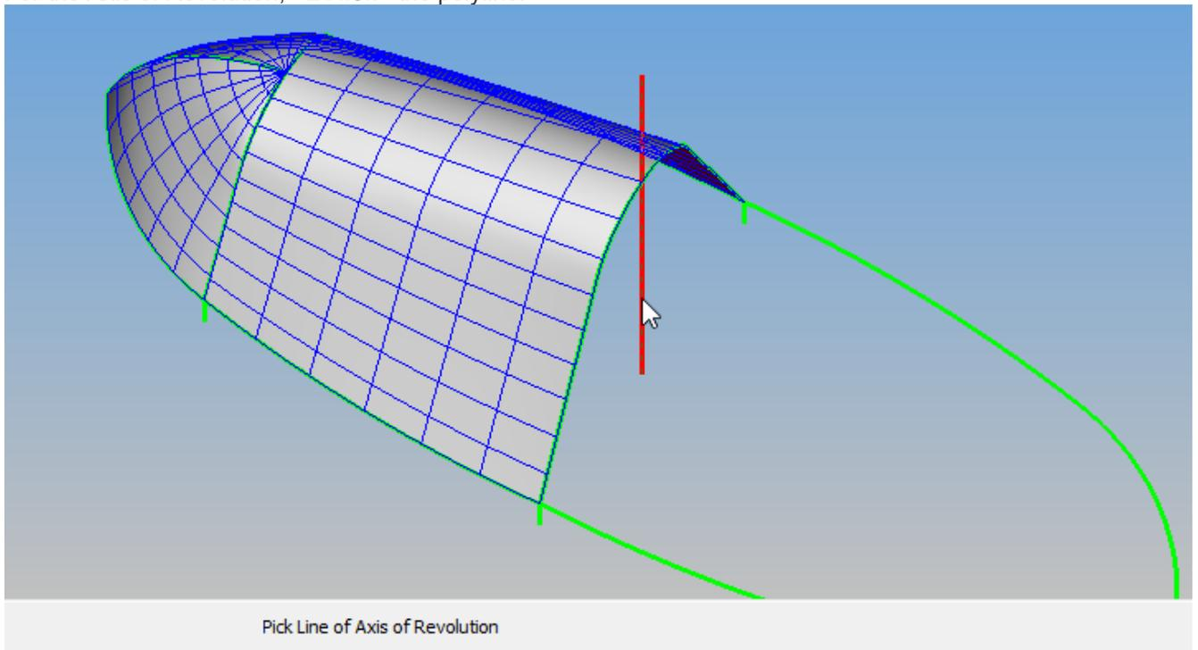
Figure 162 - Selecting the Axis of Revolution
