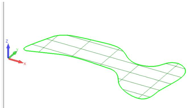
When the surface is not shaded, the parameter lines are displayed.
