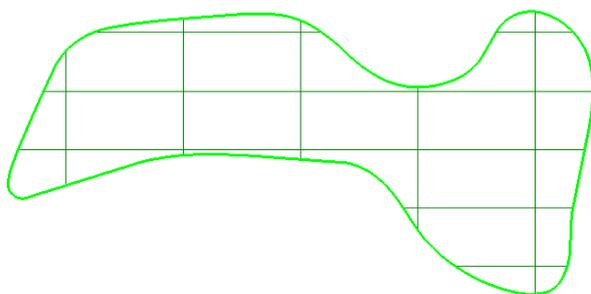
Figure 21 - Extruded surface example in wireframe
