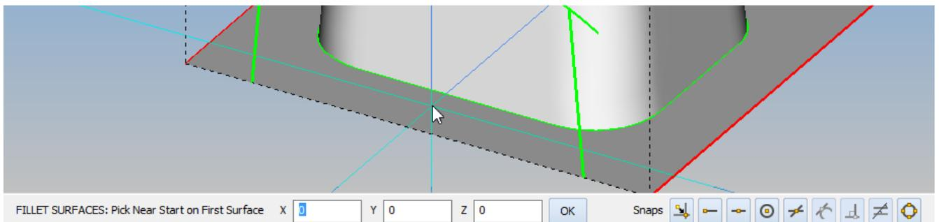
Figure 98 - Selecting the start of the fillet surface
