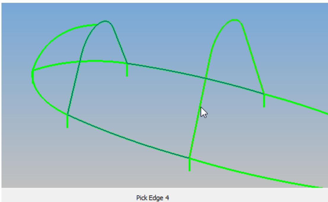
Figure 144 - Selected geometries for patch surface
