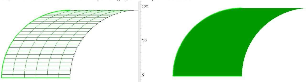
Figure 25 - Straight line sweep without rotation
