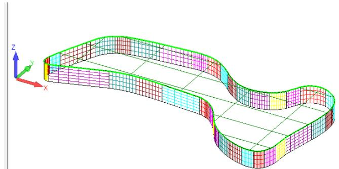
When the surface is not shaded, the parameter lines are displayed.
