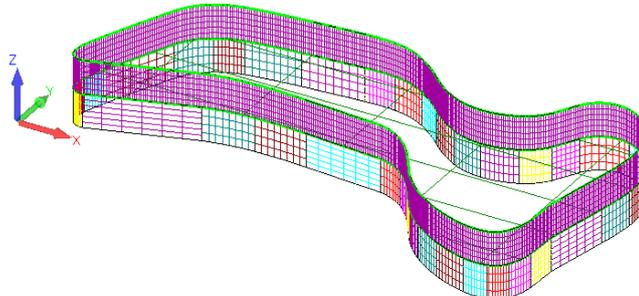
Figure 22 - Ruled surface compared to an Extruded surface
