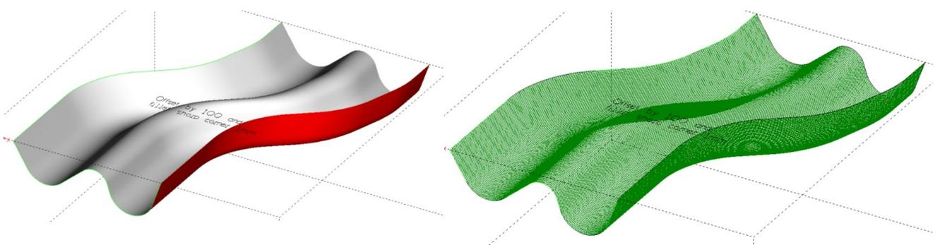
Figure 29 - Swept Surface 2 Curves completed examples
