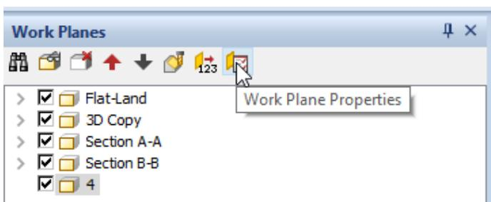
Figure 137 - Work Plane Properties command
