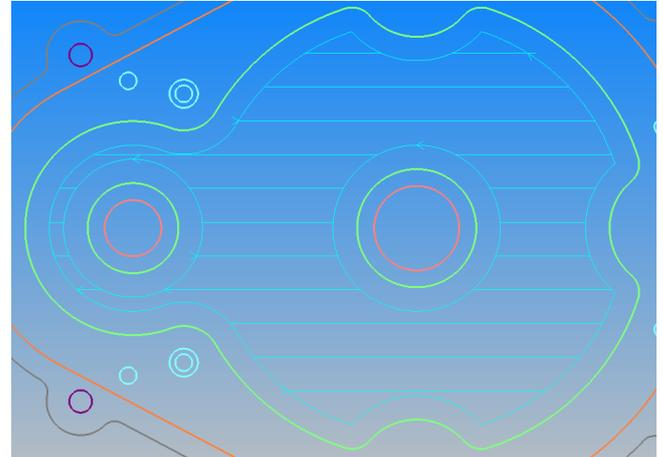
Figure 36 - Pocketing using the Linear option
