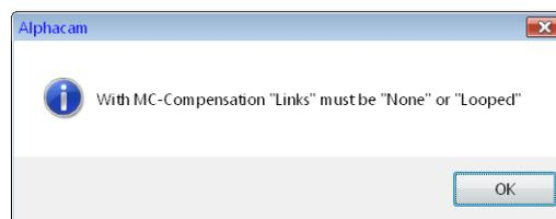
Figure 91 - Warning if using Links with the wrong Machine Compensation option
